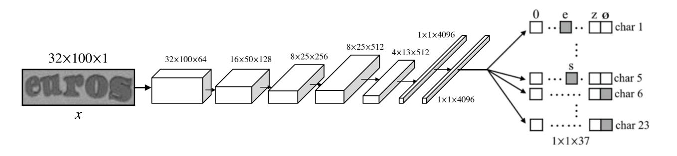
5 convolutional layers, 2 FC layers, ReLU, max-pooling 23 output classifiers for 37 classes (0-9,a-z,null)
