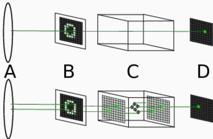
We show: If the image is illuminated coherently, and one is permitted to put an optical device in front of the sensor, one can theoretically achieve an accuracy of more than 41% on MNIST.
