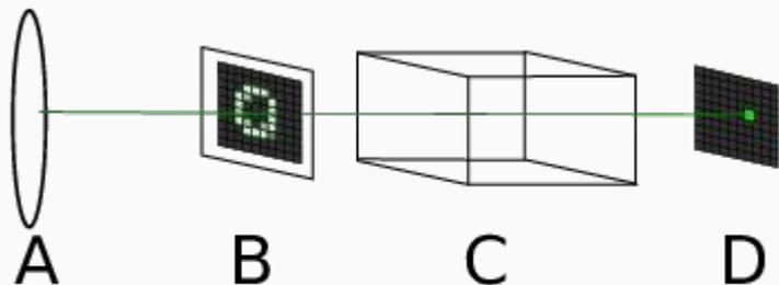
Laser illuminates screen, photon travels to single-photon detector array (SPAD), provably-optimal accuracy is MLE, *hard upper bound* of 22.96% for MNIST, "with cheating" i.e. achieved when training on the test set.
