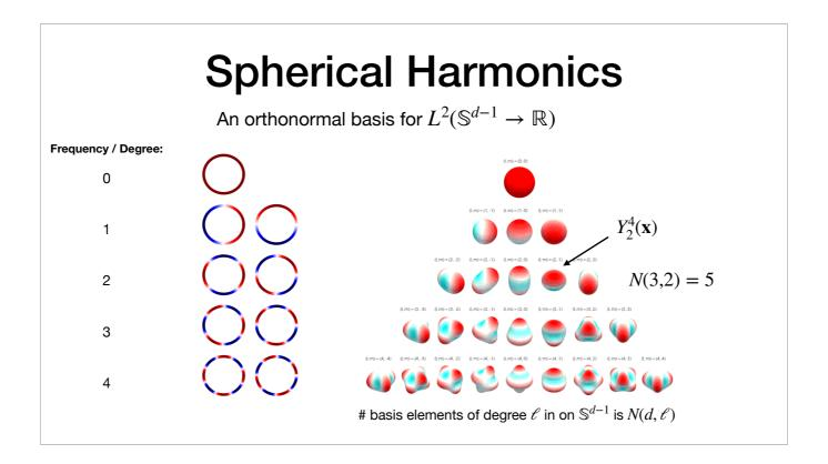
Spherical harmonics are just an orthonormal basis for functions that take a point on the sphere and output a real number. Think of these as a generalization of the Fourier basis.
