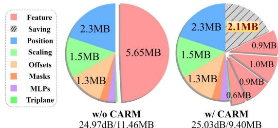
Figure 7: Breakdown analysis of different coding parts w/ and w/o our CARM for the *bicycle* scene.
