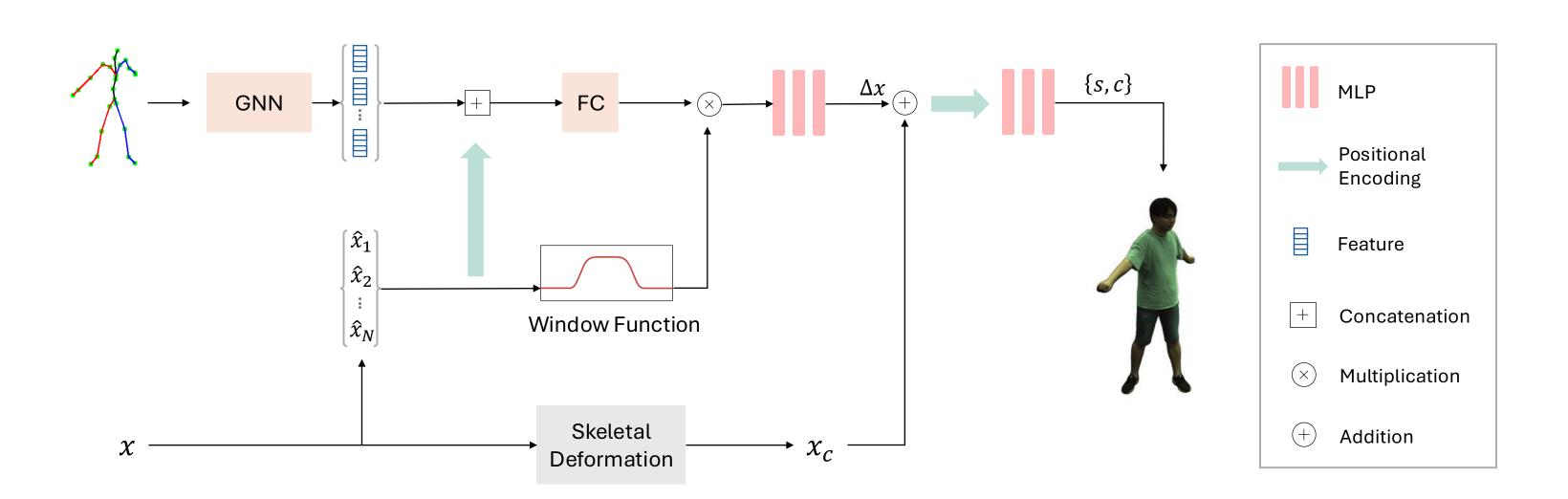
We apply inverse Linear Blend Skinning (LBS) to map a query point x from observation space to canonical space as  $x_c$  for rigid deformation modeling.
