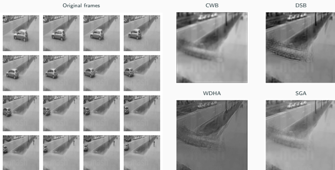
Figure 3: Left half displays 16 surveillance video frames. Right half displays their barycenters computed by CWB (top left), DSB (top right), WDHA (bottom left), and SGA (bottom right).
